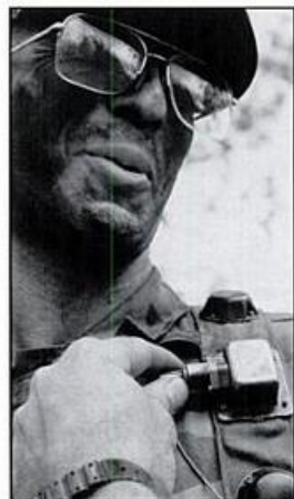
Sgt. Douglas Guy gets the alarm activated on his torso harness. Activated by a laser beam, the green controller key turns off the alarm.
